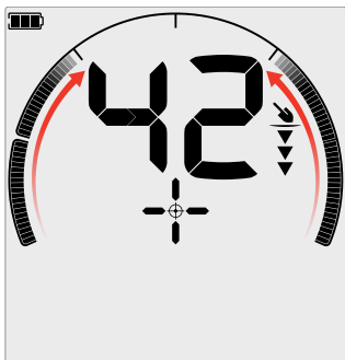
Weak/off-centre target signal: Fewer discrimination segments are On. The target is located nearer to the outside of the coil.
